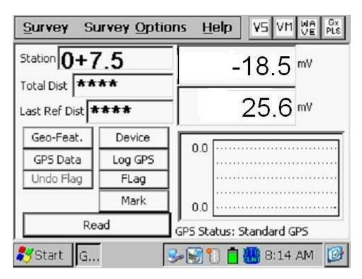
On the above example screen, the prior reading was 25.6mV and the current reading is -18.5mV. In this example, a polarity switch has been detected, which means that a gradient field has been detected.
