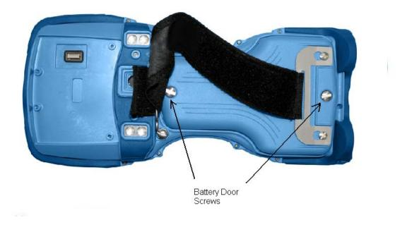
3. Unscrew both screws and remove the battery door. Both lithium-ion batteries will be revealed as shown below.
